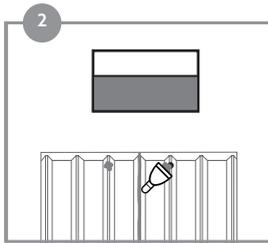
The putty must be used to cover the orifices caused by fixings and joints between panels.
