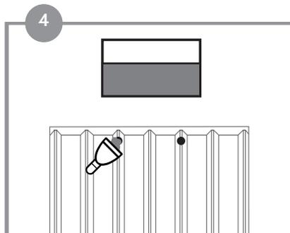
With the mixture completely homogeneous, use a spatula to cover the joints and heads of screws.
