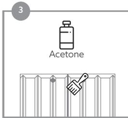
Form the texture, using acetone and a brush if using Fitmastic.
