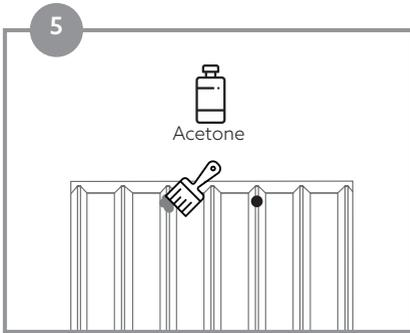
In case of using Fitmastic Fine or Fitmastic Rough, use a brush drained in acetone to give texture, imitating that of the Fitwall® panel. Lightly prod and spread with the brush until fully concealing the putty applied.
