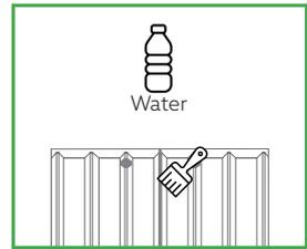
In case of using Aquafitmastic, the texture must be formed with water and a brush.
