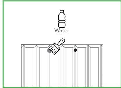
In case of using Aquafitmastic, use **water** instead of acetone to give texture, imitating that of the Fitwall® panel.
