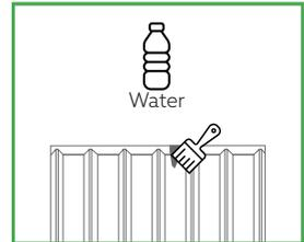
In case of using Aquafitmastic, the texture must be formed with water and a brush.
